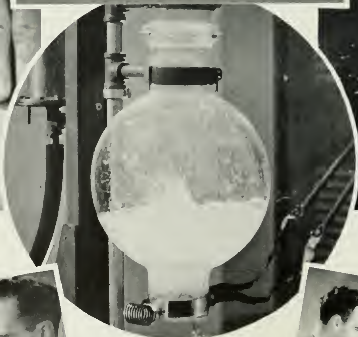
DEHYDRATING PENICILLIN BY MEANS OF RADIO-HEAT.
